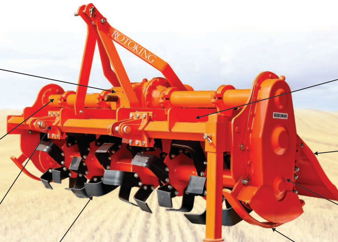
Full Housing For Better Stability Of Gear Box Assembly
